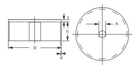
Material: Steel sheet (primed black) The protective cover is also available in stainless steel on request.
