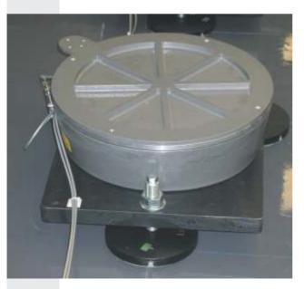
The foundation insulation using low-frequency BiAir<sup>®</sup> membrane air springs enables an optimum insulation effect. Unlike with the use of pad sets or steel springs the adjustable level of the foundation block automatically resets itself in response to load changes through the level control.
