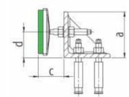
Size 1 Steel angle, Levelling element Type BNVS 115/5, 3 bolts M16 x 150, 2 anchors M16
