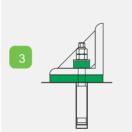
**Bolt-through** ground anchoring using insulation pads and insulation washers. The use of insulation washers prevents vibrations being transmitted through the bolt.
